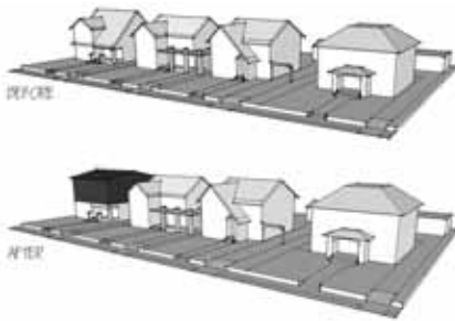
This addition disrupts the roof pattern and unique features of the home.
