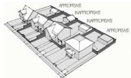
The fence arrangements in the middle two properties fortify the entire yard, obscure views of the building's features and are considered inappropriate.
